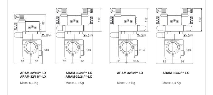
Overall dimensions refer to valves  $\ensuremath{\text{DC}}$  voltage, with connectors type 666
